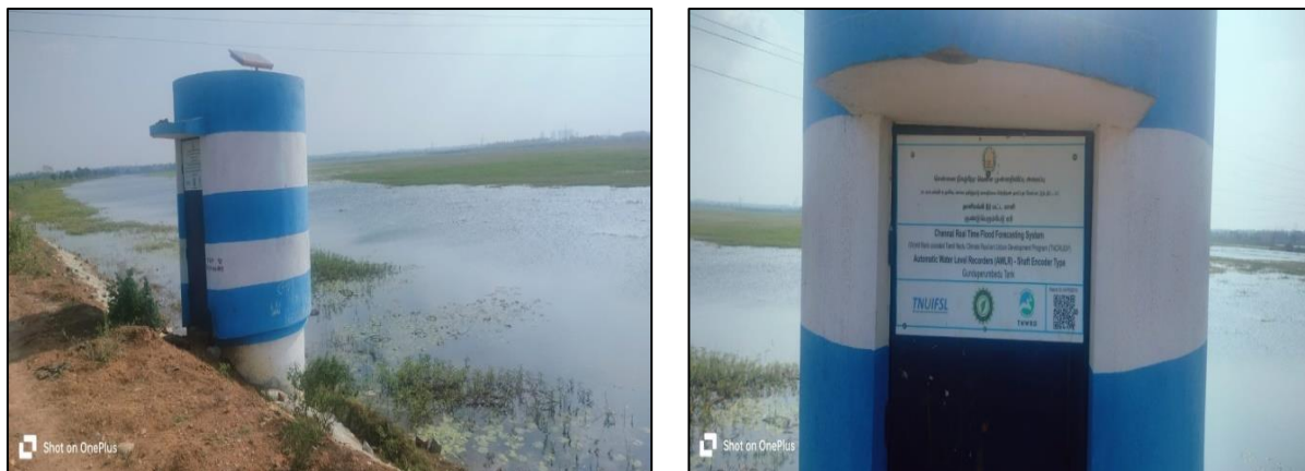
Figure 2.8: Automatic water level recorder installed at the lake
